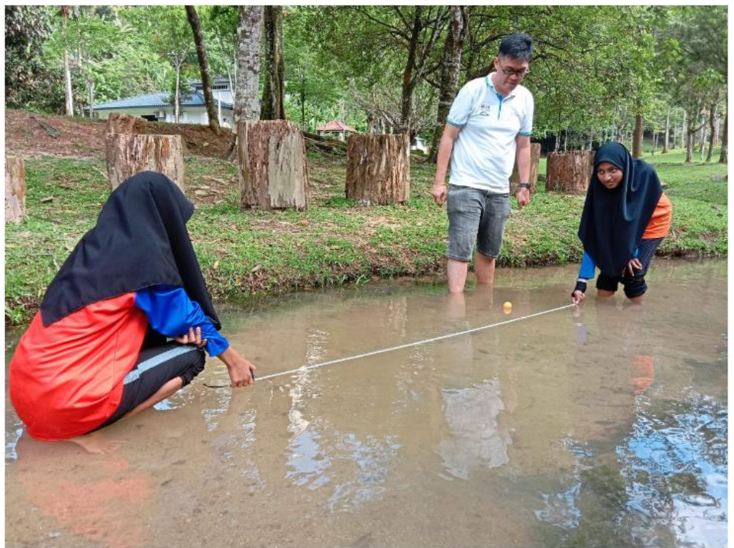
Hong guiding two students to measure river water velocity with a measuring tape and an orange ping pong ball.
